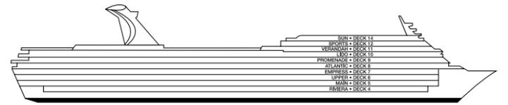
Gross Tonnage: 70,367 Length: 855 Feet Beam: 103 Feet Cruising Speed: 21 Knots
